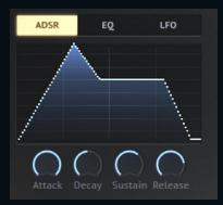
**Attack -** Adjusts the initial time it will take the envelope to reach its maximum level after it has been triggered. Ranges from 0 ms to 15 seconds.
